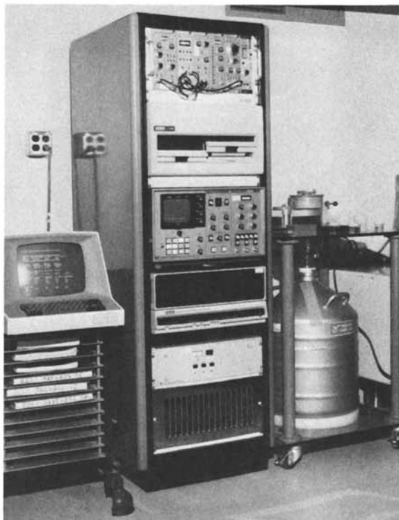
Figure 8. U solution assay system (USAS), a high-resolution gamma ray system for the measurement of U solutions at LASL's U recovery plant
