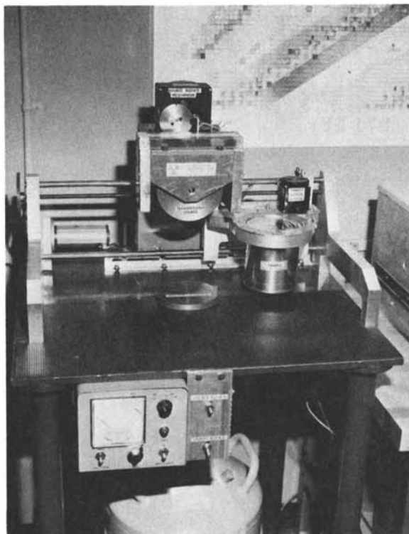
Figure 11. Can scan, a high-resolution K-edge densitometry device for the measurement of Pu-bearing ash in cans
